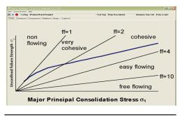
Figure 3: Graph Shows Standard Flow Function Test Data and Regions of Flow Behavior
