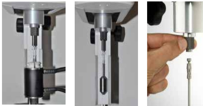
Figure 1: Concentric/coaxial cylinder accessory with easily-locking coupling (a). Spindle immersed in sample chamber, held in cooling/heating jacket (b). Spindle hanging from coupling (c). Coupling collar lifted up to allow spindle insertion or removal
