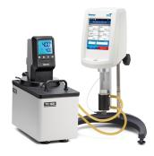
(See Figure 3) This measurement can be equated with the startup torque in a motor that drives the mixing pump on the production floor or the squeezing force applied by the end user to get the product out of the tube. So for more viscous products, the rheometer may offer an advantage in terms of additional measurements that could prove useful.
