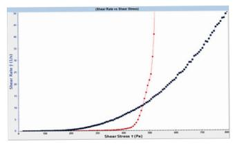
Figure 3: Controlled Stress Test Provides Yield Stress Value for Start of Flow Figure 4: Flow Curve Shows Viscosity vs. Shear Rate Behavior
