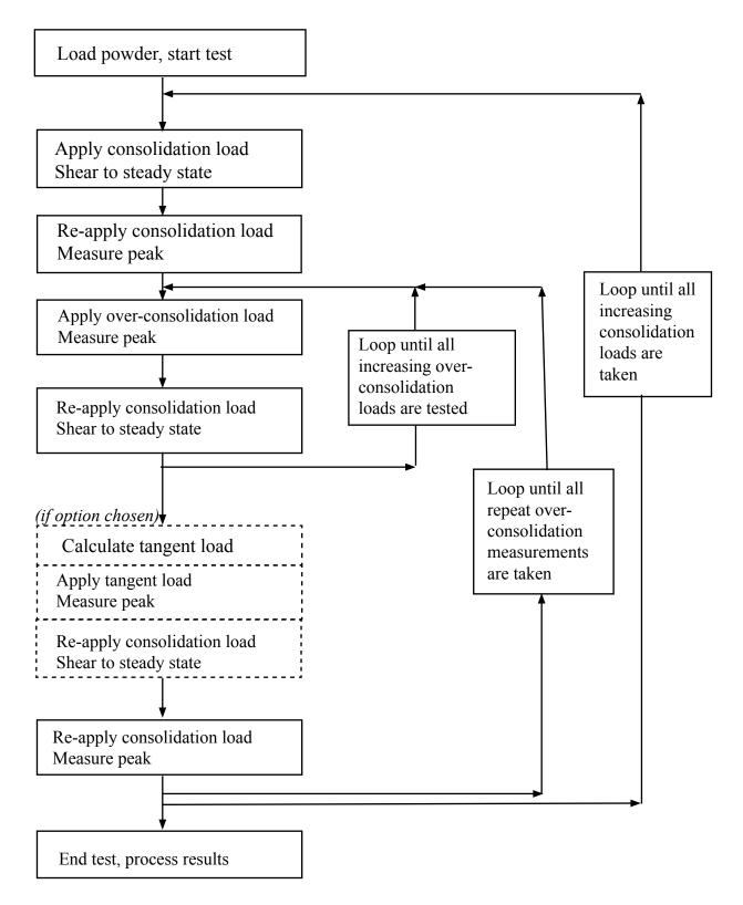
Figure IV-8: Flow Function Test Algorithm.
