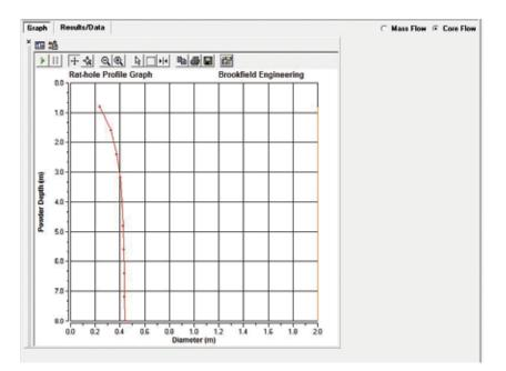
Figure IV-24: Powder Depth vs. Rat-Hole Diameter Graph
