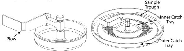
Figure III-6a: Inner Catch Tray with Shaping Blade in Position to use Curved Profile
