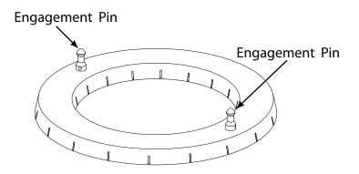
Figure III-4a: Top Side of Lid Showing Engagement Pins
