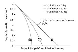
Figure A-6: Stress distributions in vertical walled vessels
