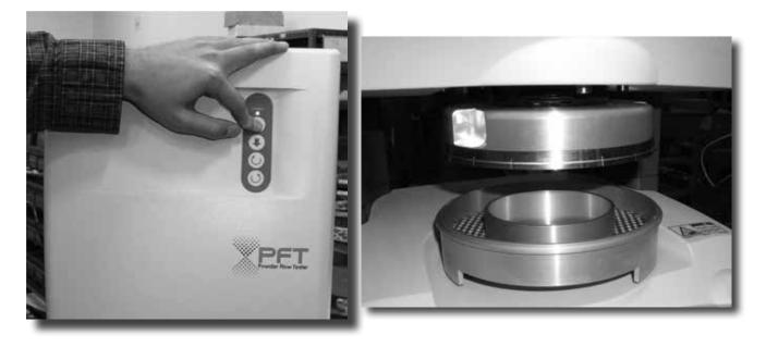
4) Place the circular foam insert (PFT-101 for 6" Trough and PFT-106 for 5" Trough) into the Trough. Remove the Trough to accomplish this, if necessary, from the PFT. Install the Trough on the PFT.
