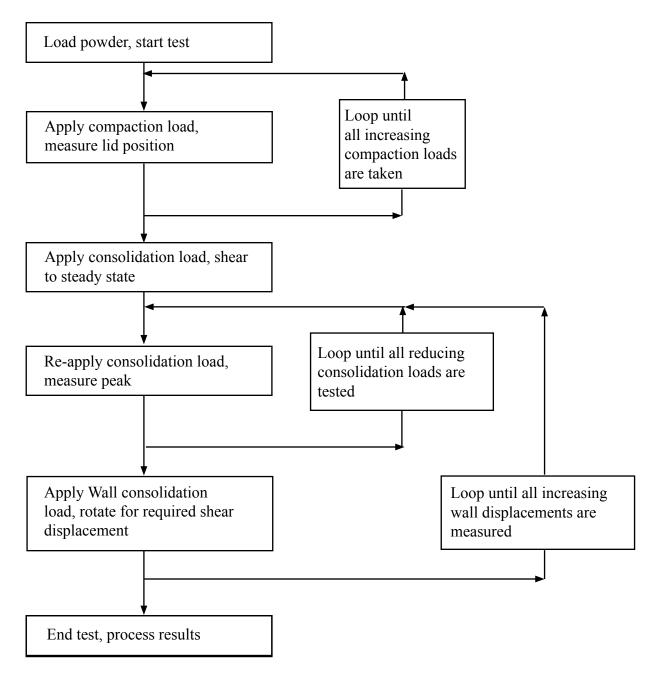
Figure IV-10: Wall Friction Test Algorithm
