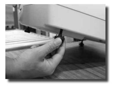
2) Ensure that the Vane Lid (Part Number PFT-500 for 6" Lid or Part Number PFT-515 for 5" Lid) and Trough (Part Number PFT-400 for 6" Trough or Part Number PFT-405 for 5" Trough) are installed on the PFT. This is necessary in order to lock the suspension system inside the instrument so that movement cannot take place during transport.
