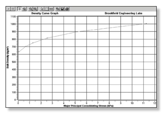
• Bulk Density Curve Test data shows one density curve including initial fill density.
