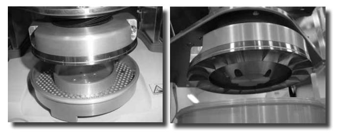
3) Raise the Vane Lid to its uppermost position by pressing the up arrow.
