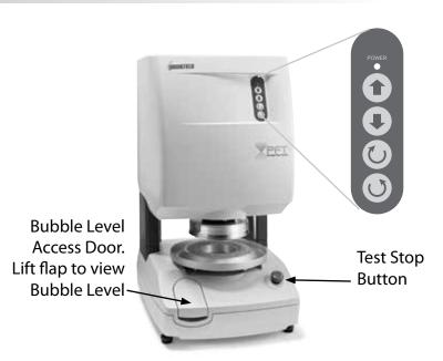
Figure I-3: Control keys for standalone mode
