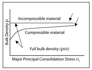
Figure A-9: Bulk density curve
