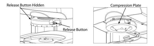
Figure III-4b: Release Buttons
