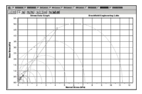
Figure IV-15: Stress Data Graph for Flow Function Test
