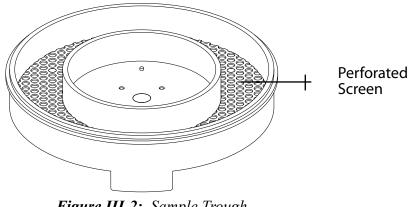
Figure III-2: Sample Trough
