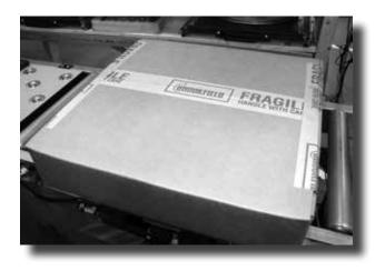
17) Place the accessory carton (PFT-PACK1) on top of the top foam packaging piece. If you do not have the accessory carton, please contact Brookfield for replacement parts. If the accessory carton is not used, damage to the instrument may occur.
