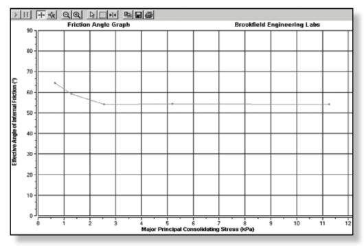
Figure IV-20: Friction Angle Graph for Flow Function Test
