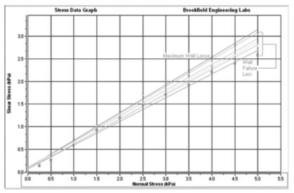
Figure IV-16: Stress Data Graph for Wall Friction Test
