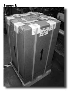
20) Apply labels which say "SHIP ONLY BY FREIGHT". These labels are included in the Repack Kit (Part Number LBL11-PFT3). Place one label on the top of the shipping carton and one on the side, see figures below.
