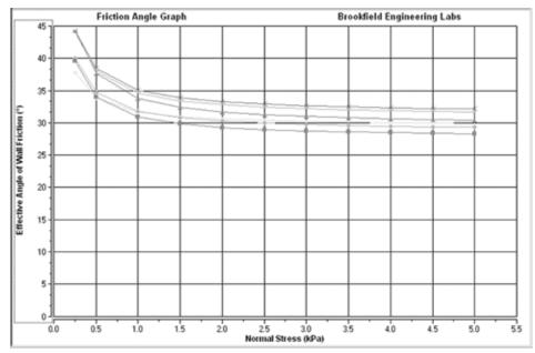
Figure IV-21: Friction Angle Graph for Wall Friction Test
