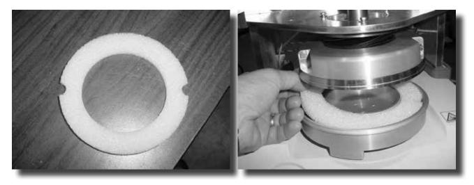
5) Press the down arrow to lower the Vane Lid until it just makes contact with the foam insert. Then press and hold the down arrow for 2 seconds. This will adjust the position of the Vane Lid so that the foam is slightly compressed. Do not hold longer than 2 seconds because this will cause further compression of the foam insert, which is not desired.
