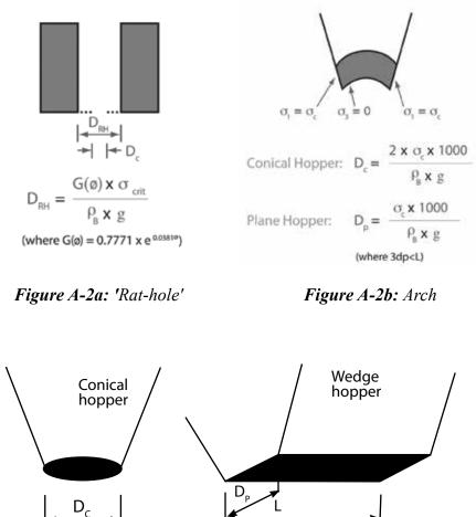
Figure A-3a: Conical hopper Figure A-3b: Wedge (plane) hopper
