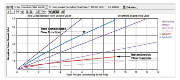
Figure IV-18: Time Consolidation Test Graph
