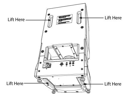
Figure I-4: Back View of Hand Hold locations
