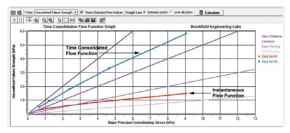
Figure IV-25: Time Consolidated Flow Function Test Graph
