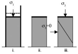
Figure A-4: Uniaxial unconfined failure test
