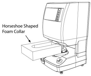
Figure I-5: Removal of foam collar
