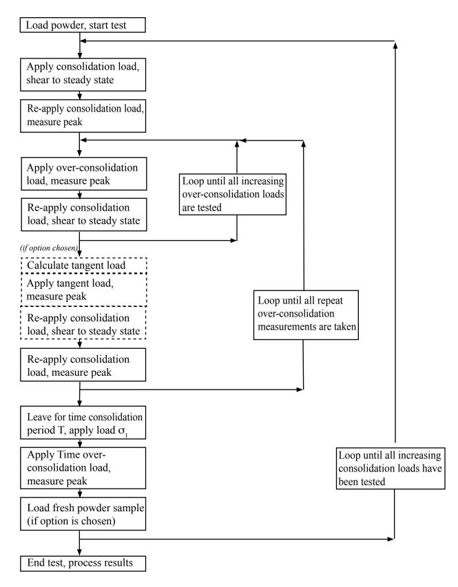
Figure IV-9: Time Consolidated Flow Function Algorithm
