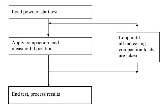
Figure IV-11: Bulk Density Test Algorithm
