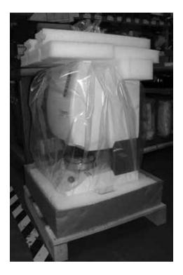
14) Slide the outer carton box (PFT-PACK2) over the PFT and insert <u>between</u> the outer carton packaging kit and the bottom foam packaging piece.
